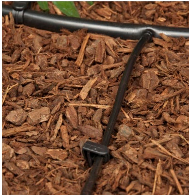
Once the 1/2" poly tubing has been installed, then the 1/4" micro tubing can be connected. First attach the micro tubing to the 1/4" barb (or 1/4" tee), then use the punch to make a hole in the 1/2" poly tubing and then insert the barb into the hole. Install a dripper or micro-sprayer at the end of the micro-tubing and use it as a feeder line to reach remote plants or clusters of plants that are away from the main 1/2" tube.
